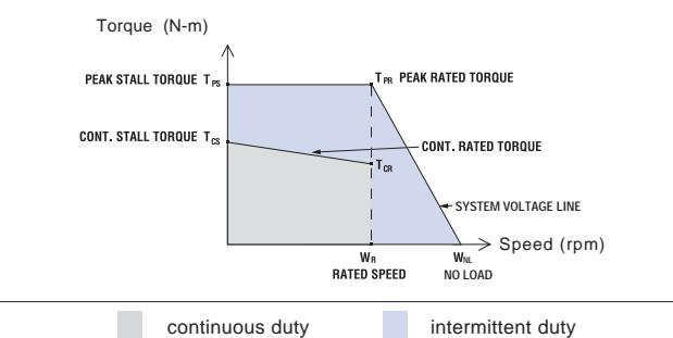
System torque/speed information on the following pages is designed to help you select the optimum brushless servo motor/controller combination.
